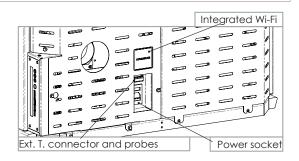
It is compulsory for the system to be grounded and have a differential switch in compliance with legislation in force. Furthermore, ensure the socket is compatible with the type of plug on the power cable used.
