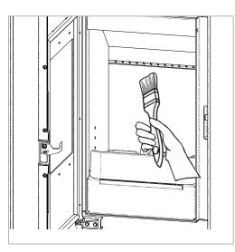
Vacuum the cast-iron combustion plate and the fire pit, fpaying attention not to knock the nozzle of the vacuum cleaner against the vermiculite.
