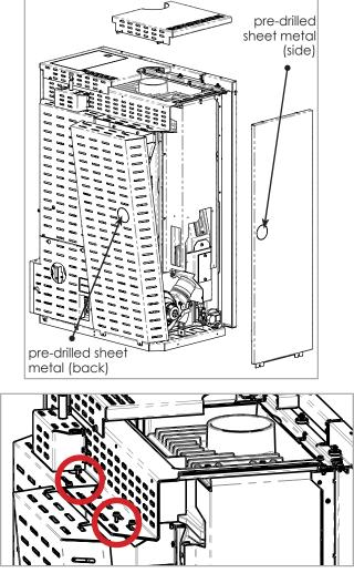
Fasten the canalization kit using the 5 screws (highlighted) already present in the stove
