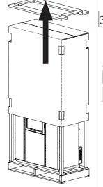
Toremove the appliance from the pallet, you can remove the two screws placed under the pallet (13 hex key) to release the appliance from the wooden base. Position the product and proceed with
