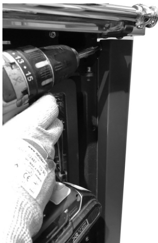
Fig. 40 - Attach the side panels onto 2 screws
