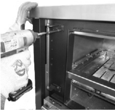
Fig. 23 - Remove the brackets
