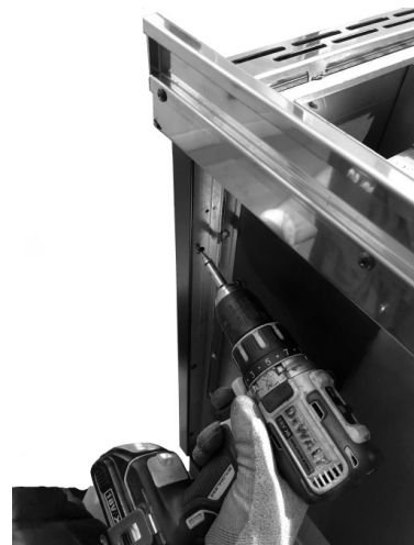
Fig. 41 - Fasten the side panels onto 3 screws
