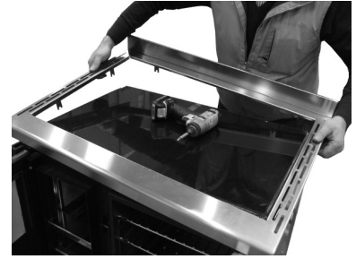
Fig. 73 - Remove the top
