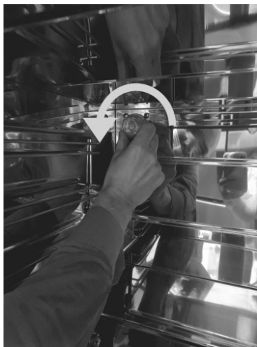
Fig. 61 - Unscrew the lamp cover
