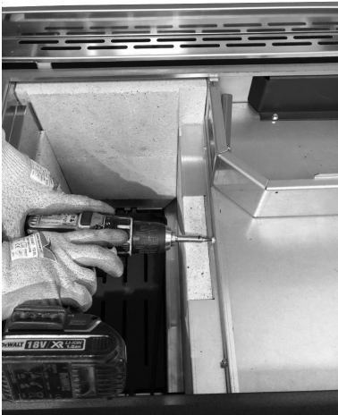
Fig. 66 - Unscrew the profile
