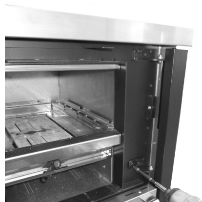
Fig. 27 - Fix the lower bracket
