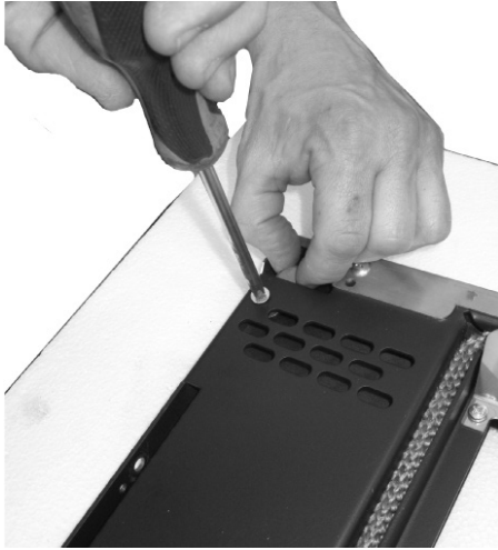
Fig. 34 - Fix the door locking screw
