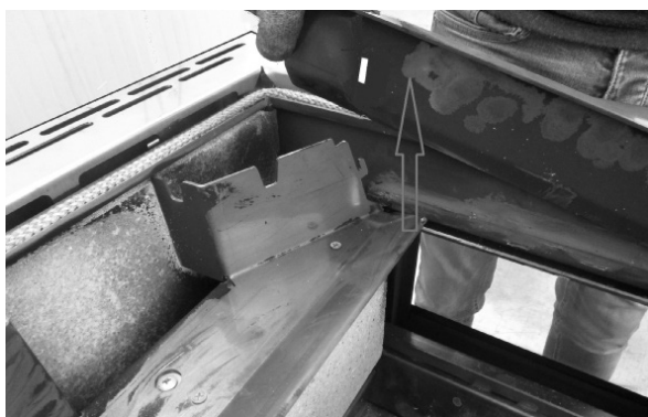
Fig. 62 - Remove the front profile
