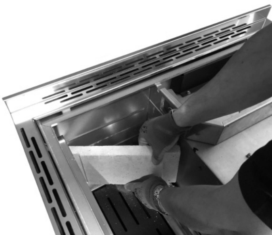
Fig. 69 - Remove the refractory material 2
