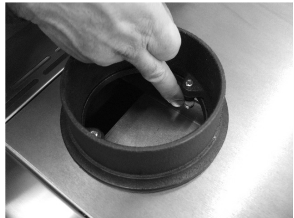
Fig. 46 - Fasten the stub pipe
