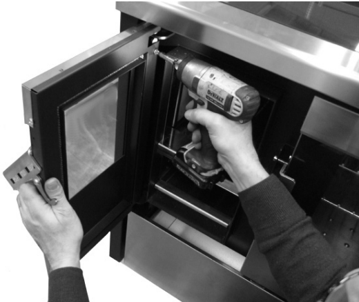
Fig. 74 - Undo the screw
