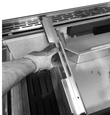
Fig. 67 - Remove the profile
